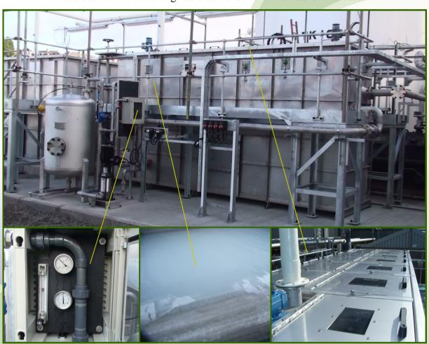
White water is produced using a venture and gap meter to reduce operating cost.
