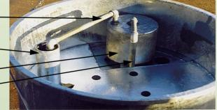
Quickstrip back entry nozzle rodding caps are fitted to allow easy removal of trash and cleansing of nozzle using standard HYCOVER rodding brush.
